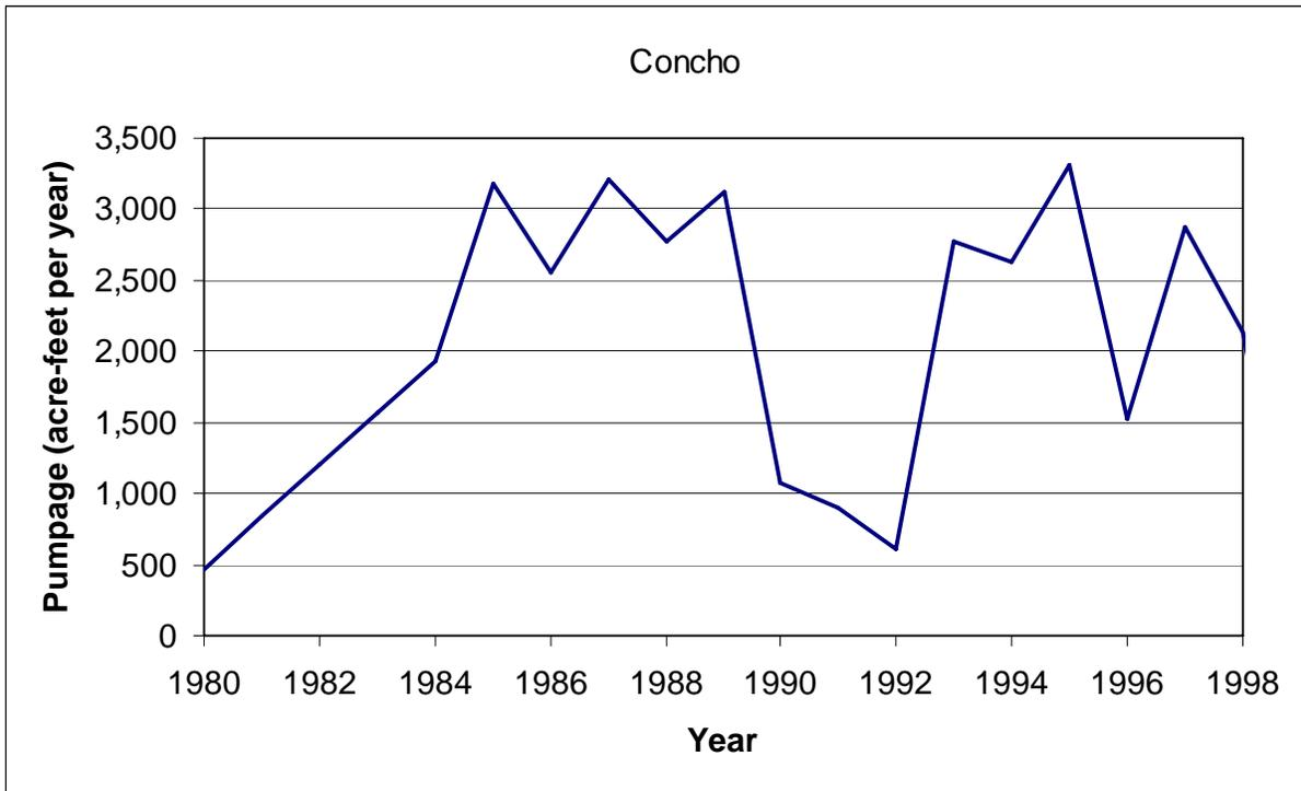
Figure A-2- Pumpage in Concho County included in the model for the Lipan Aquifer.
