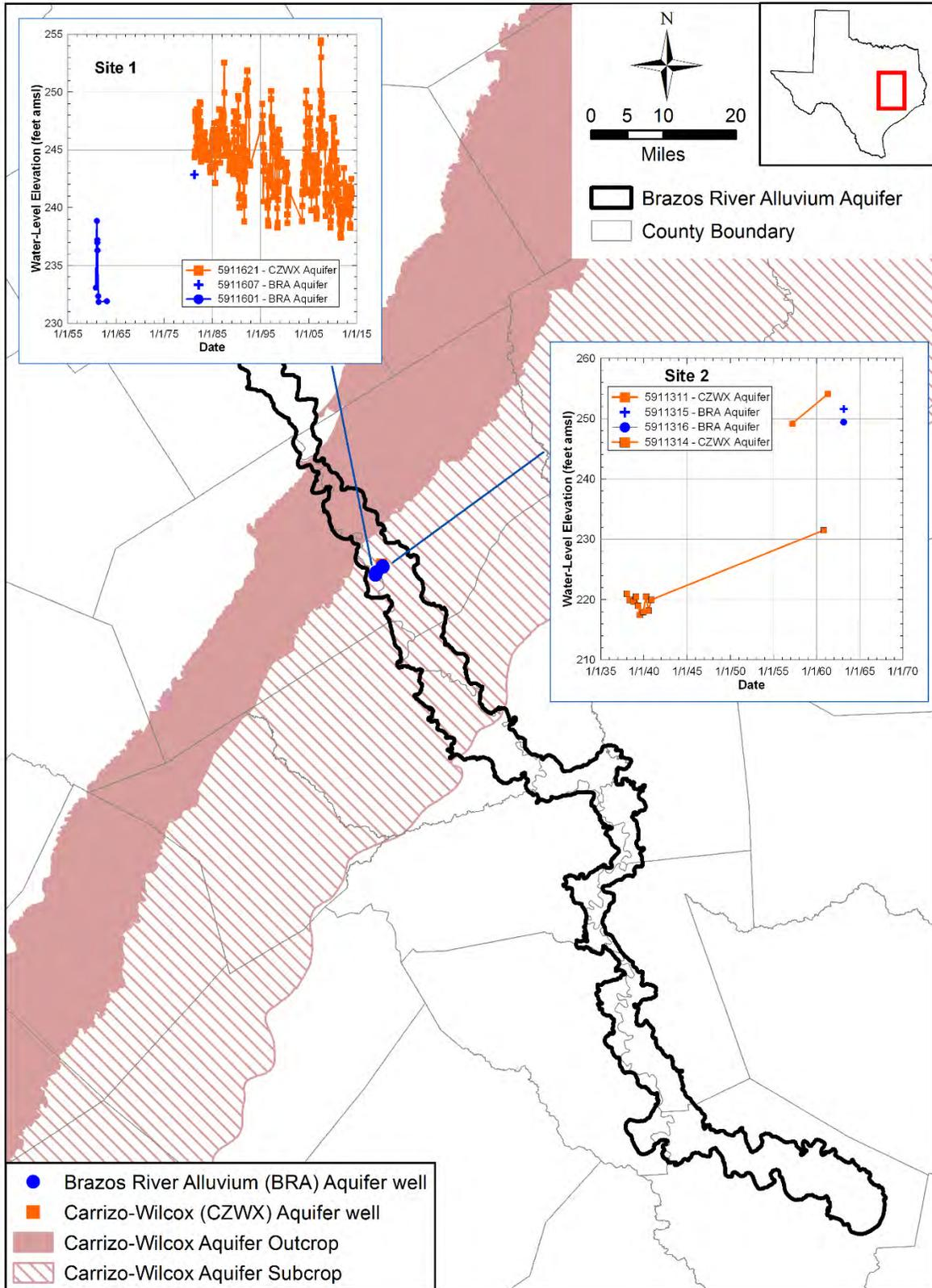
Figure 4.2.24 Comparison of water-level elevations in feet above mean sea level in the Brazos River Alluvium Aquifer and the underlying Carrizo-Wilcox Aquifer.
