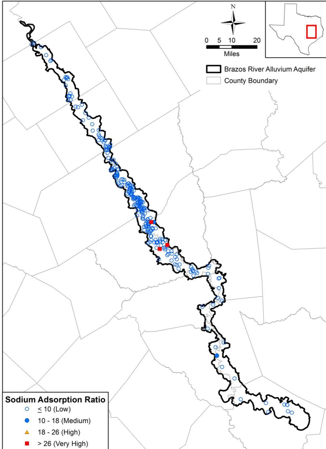
Figure 4.7.7 Sodium hazard in the Brazos River Alluvium Aquifer (TWDB, 2014f).
