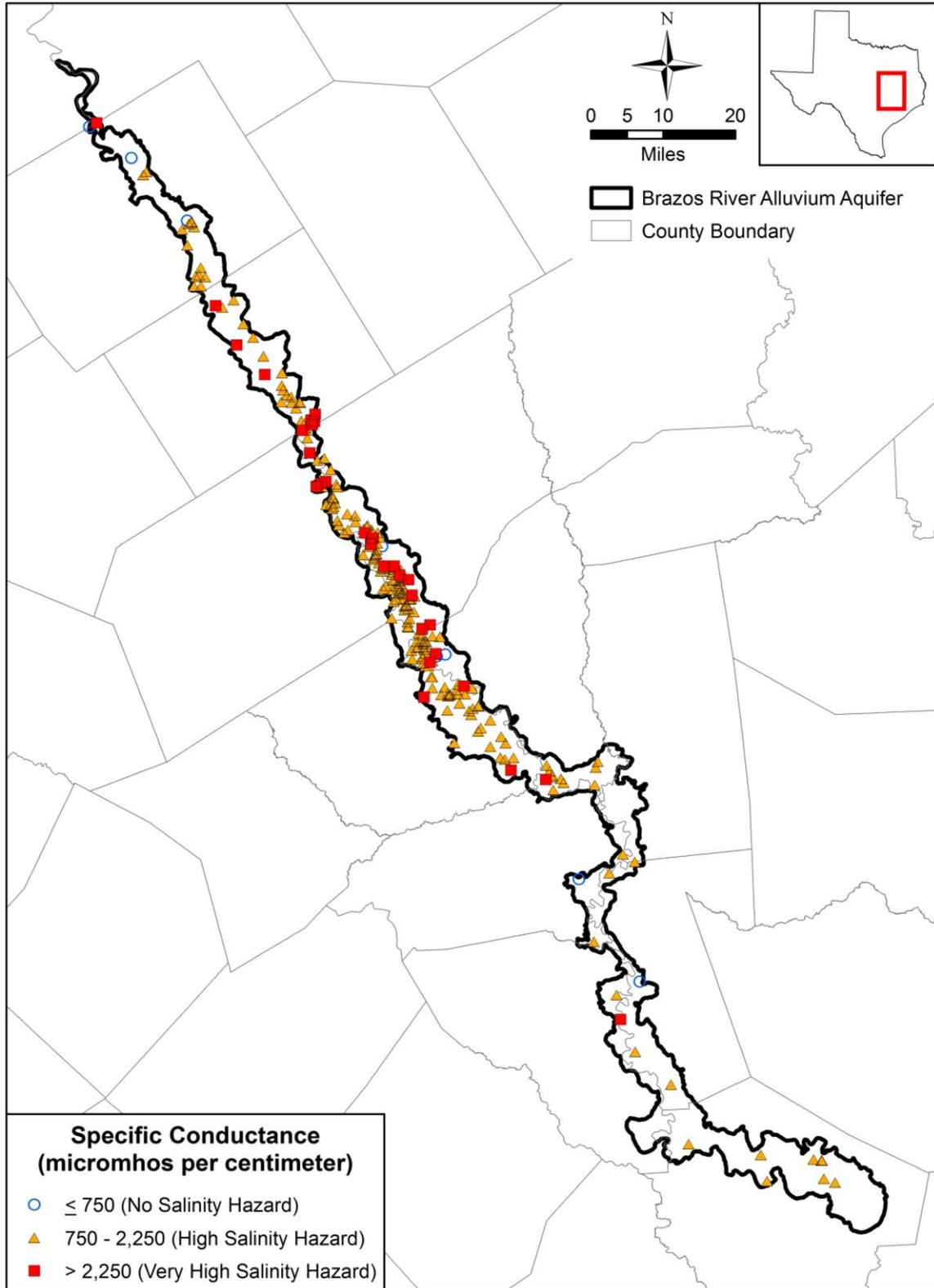
Figure 4.7.6 Irrigation salinity hazard in the Brazos River Alluvium Aquifer (TWDB, 2014f).
