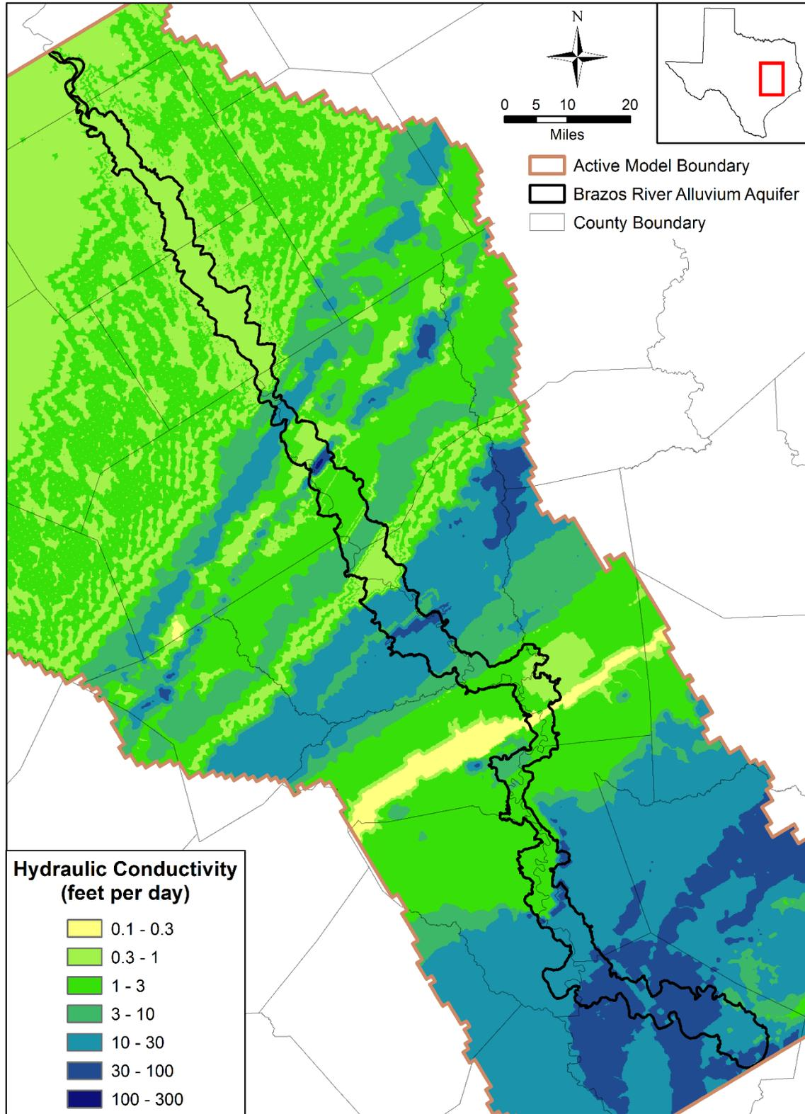
Figure 4.5.7 Horizontal hydraulic conductivity distribution for geologic units underlying the Brazos River Alluvium Aquifer.
