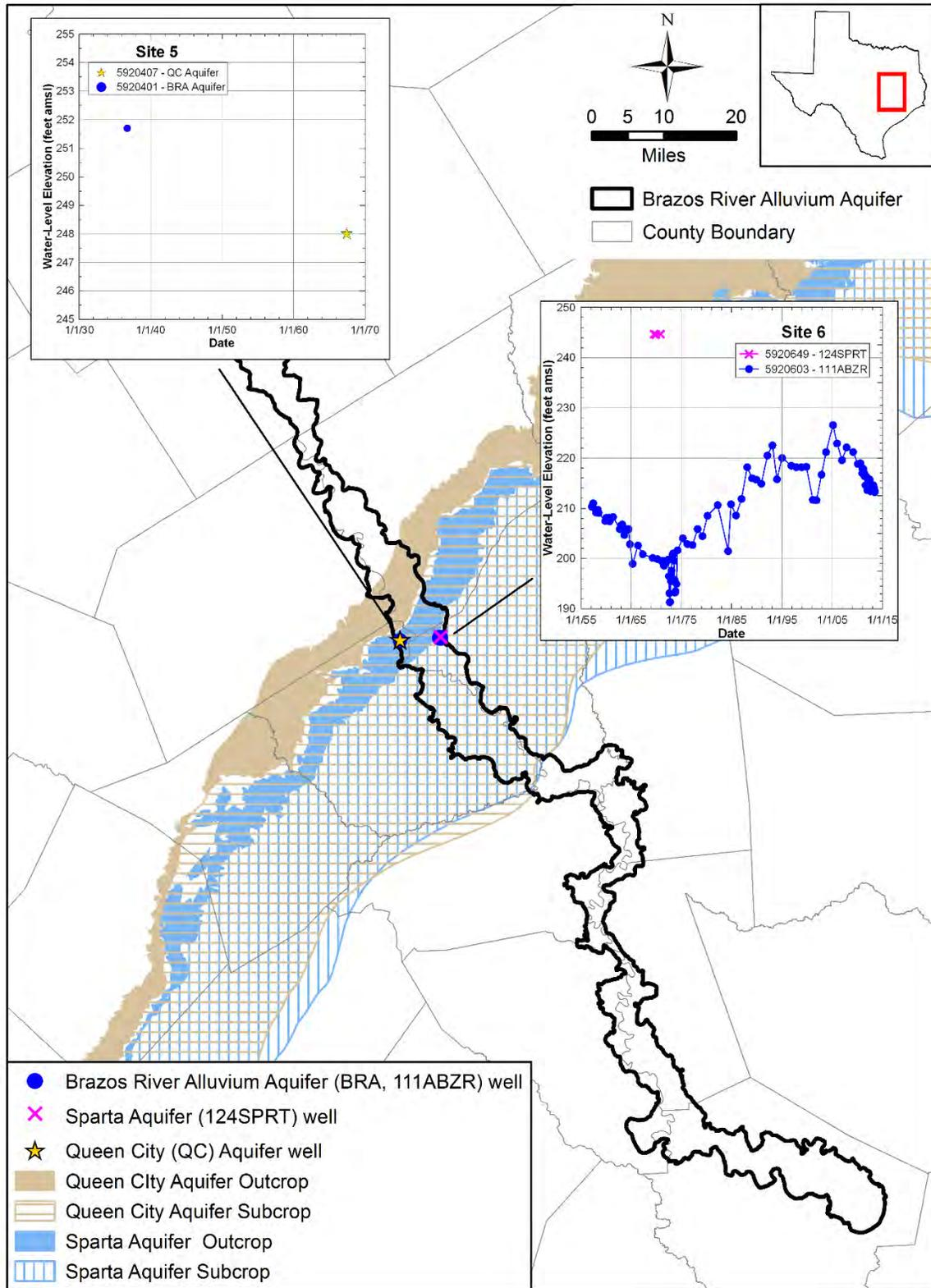
Figure 4.2.25 Comparison of water-level elevations in feet above mean sea level in the Brazos River Alluvium Aquifer and the underlying Queen City and Sparta aquifers.
