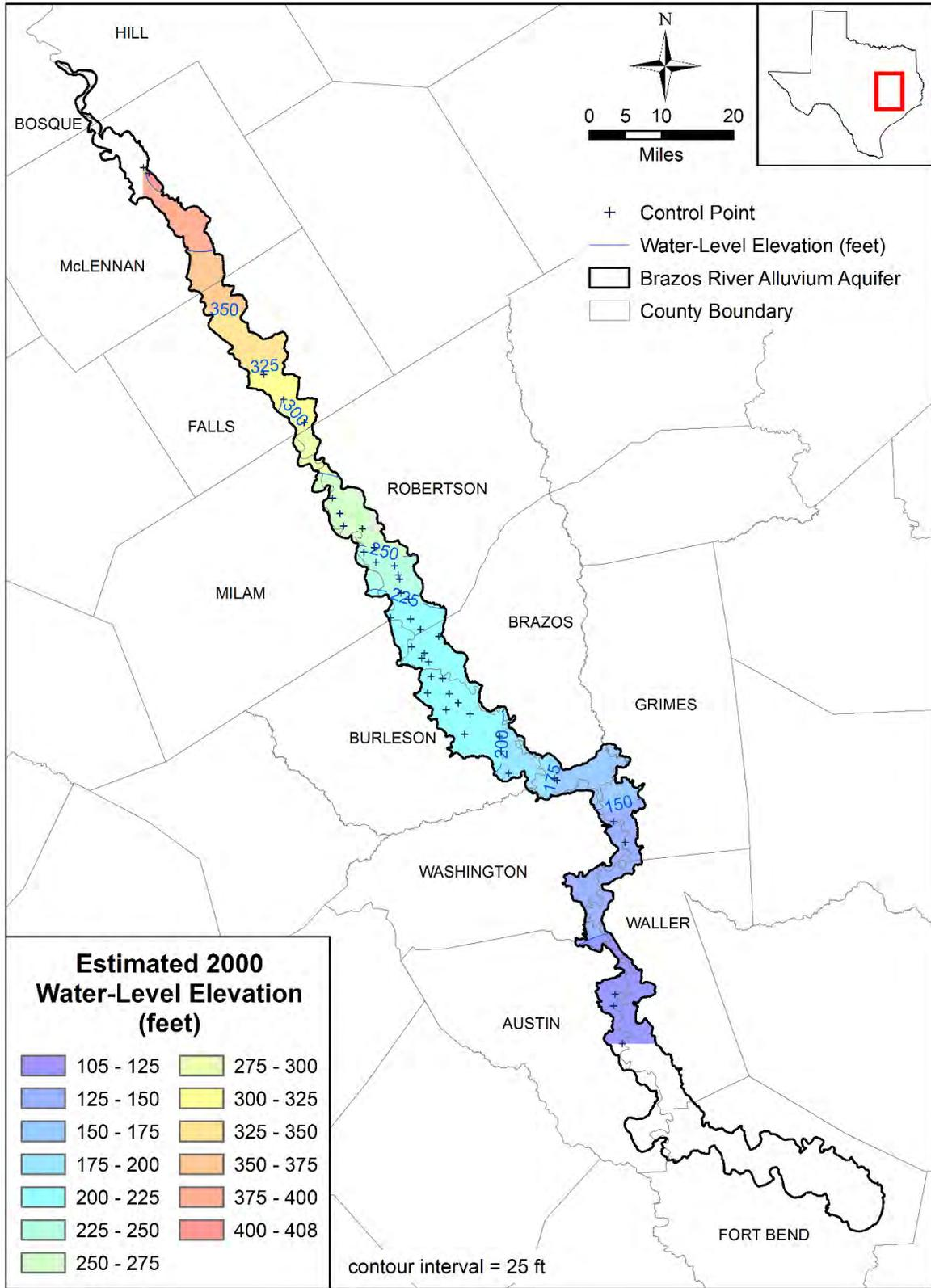
Figure 4.2.20 Estimated water-level elevation contours in feet above mean sea level in the Brazos River Alluvium Aquifer in 2000.
