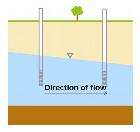
Hydraulic conductivity – A physical property of the geologic media representing its ability to transmit water (related to permeability and transmissivity)
