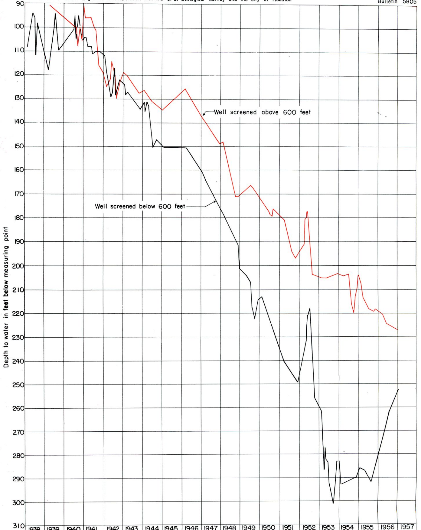
FIGURE 17. - Changes in water levels in a shallow well and a deep well in the eastern part of the ship-channel subarea.
