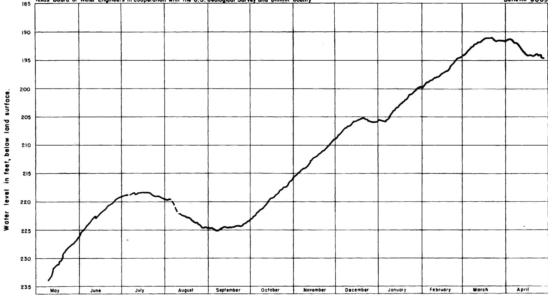
FIGURE 10.—Daily water levels in well N9-24 for the period May 9, 1957 to April 27, 1958.
