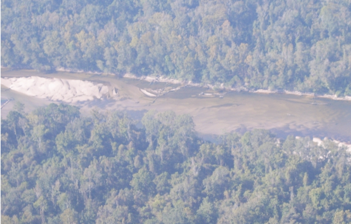
Figure 7. Mid-channel bars in a straight reach of the lower Sabine River. Photographic examples of all major bar types are given in Appendix B.
