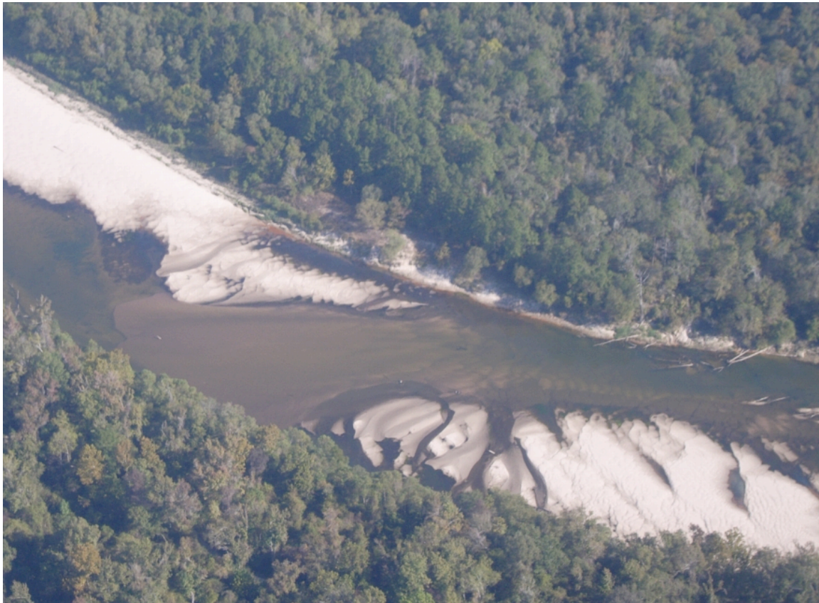
Figure 12. Linguoid bar formed due to constriction between two closely-spaced alternate side marginal bars.
