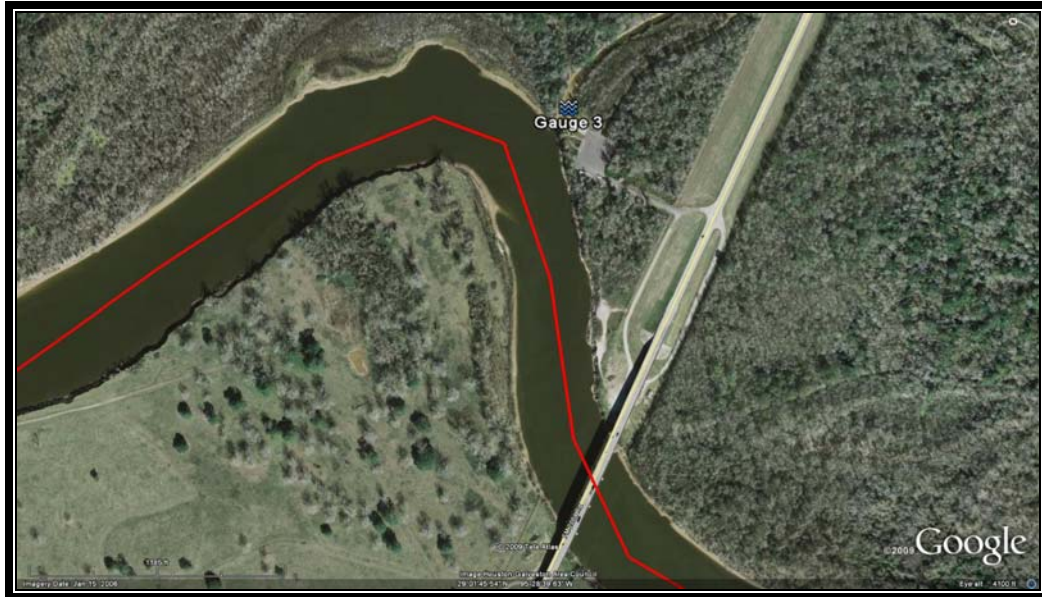
Figure 9. Showing location of Hobo water level logger at Gauge 3.
