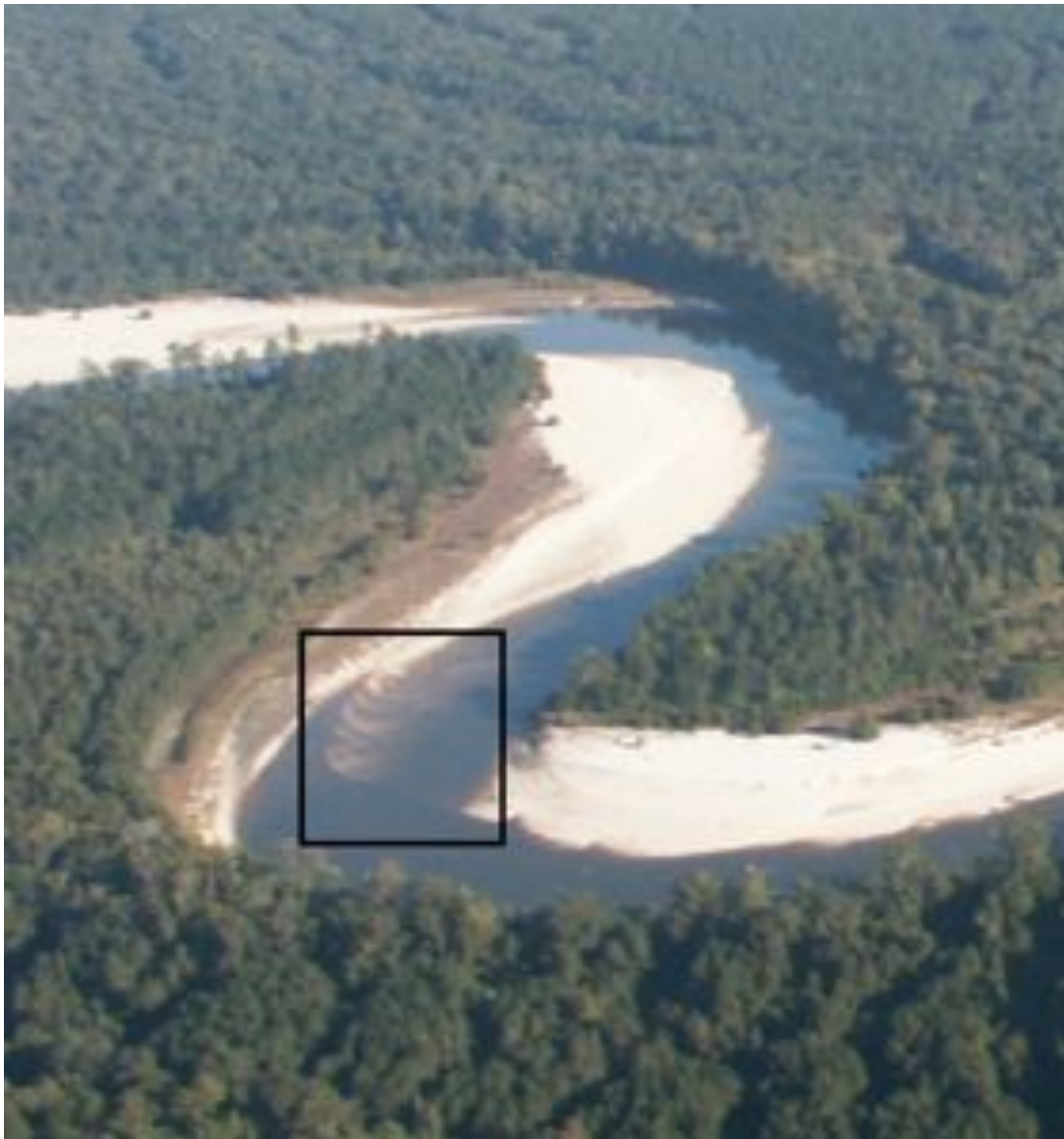
Figure 3. Low-level aerial photograph from October, 2007. The box shows cusped bedforms on an extender type of connector bar.
