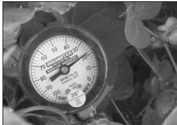
Figure 10: (Top) Tensiometers installed at the demonstration site. (Bottom) Vacuum gauge of the tensiometer. A values of 50 indicates the need for irrigation and a value of 20 indicates saturated conditions.
