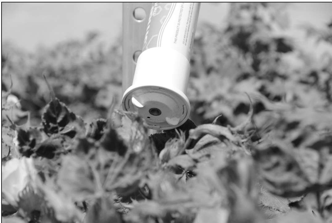
Figure 7: SmartField sensor in the demonstration field. (Photo by Nithya Rajan)
