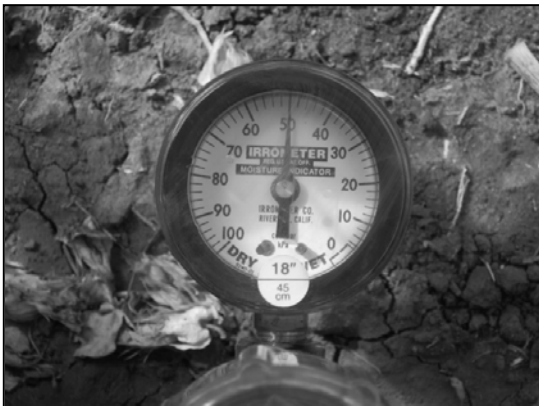
Figure 10: (Top) Tensiometers installed at the demonstration site. (Bottom) Vacuum gauge of the tensiometer. A values of 50 indicates the need for irrigation and a value of 20 indicates saturated conditions.
