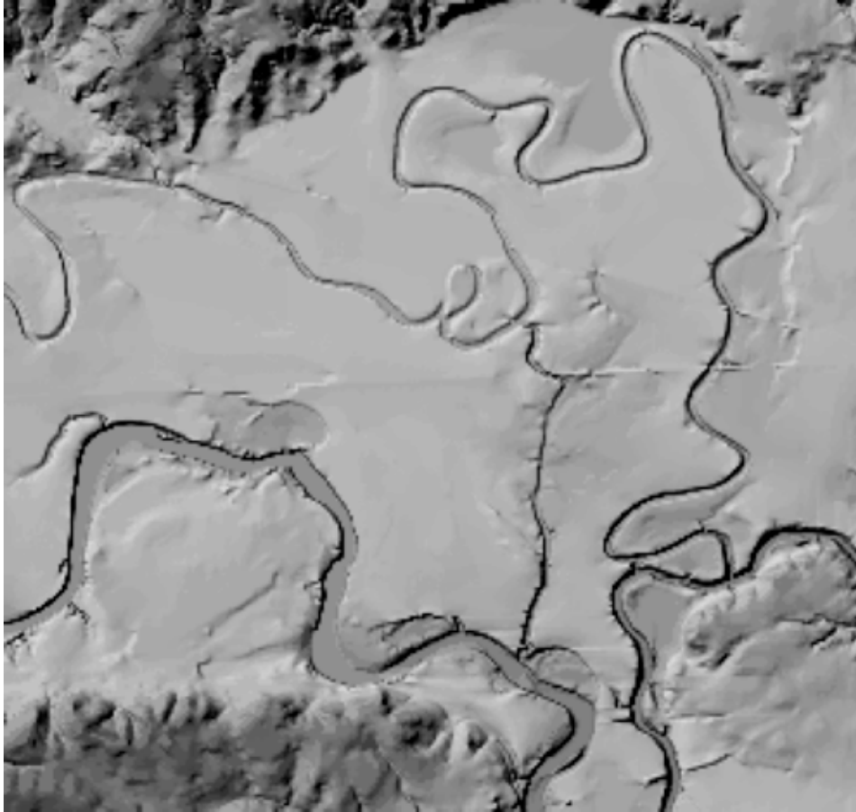
Figure 15. Shaded relief of the Big Creek area along the Brazos River between College Station and Navasota. Big Creek (a former Brazos River channel) is the primary source of water for many floodplain depressions.
