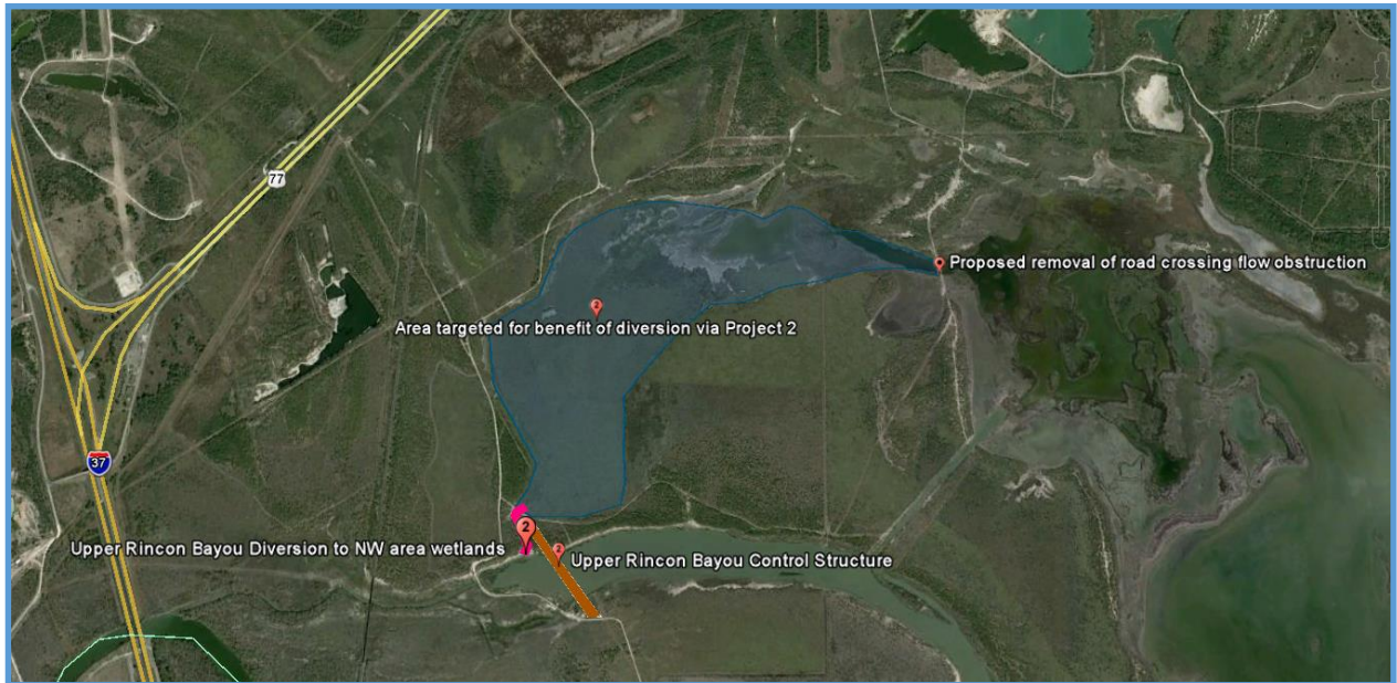
Figure 3.1.1-2: Project #2 -- Upper Rincon Bayou Diversion to High Marsh/Wetlands N. of Rincon Bayou
