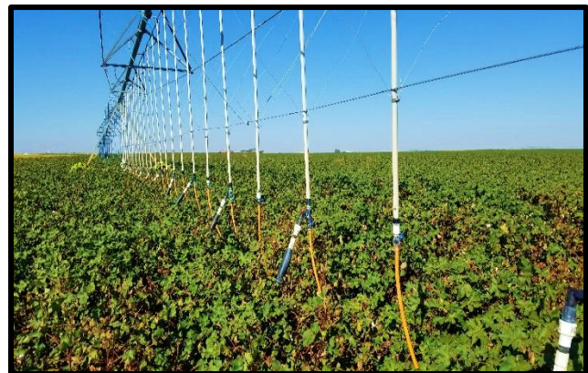
Standard irrigation pivot modified with dragon line drip system
