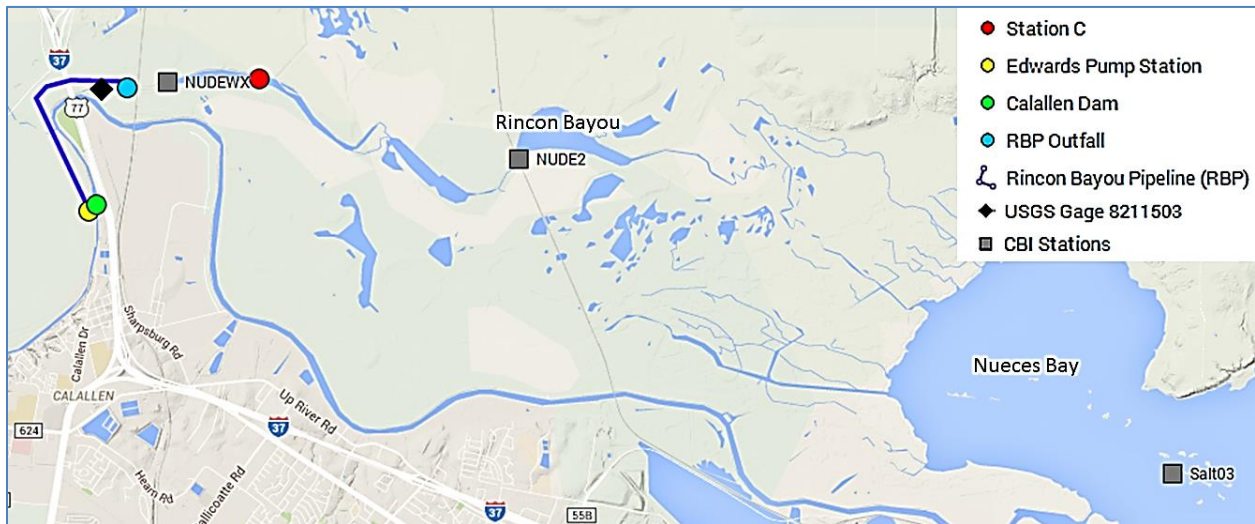
Figure 3. Map of station locations for measuring flow, salinity, and weather in Rincon Bayou.
