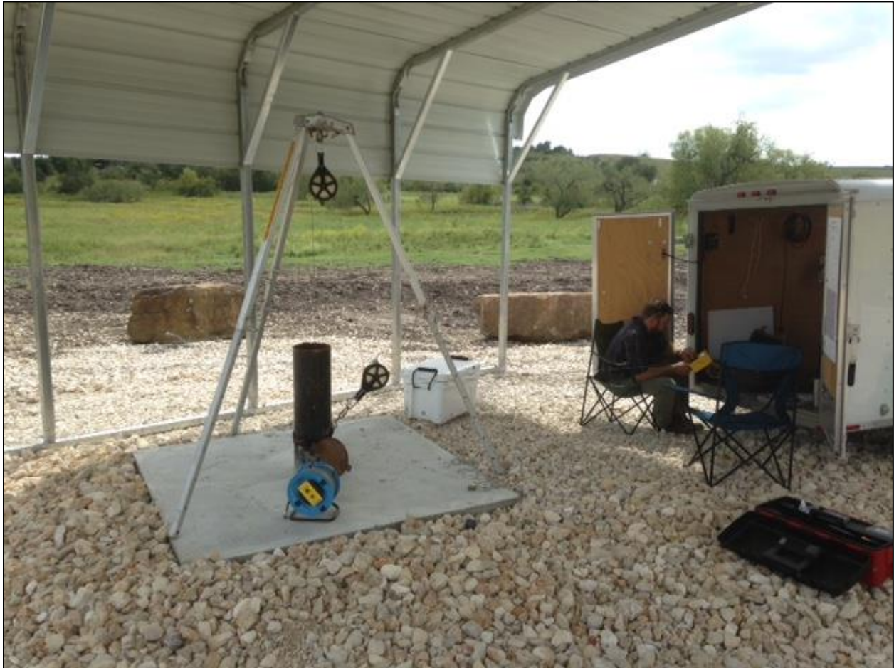
Figure 15. Photograph showing equipment during measurement of a profile of water-level data. The trailer contains a winch that lowers the measurement instrument into the well. Photo taken 10/6/2016.
