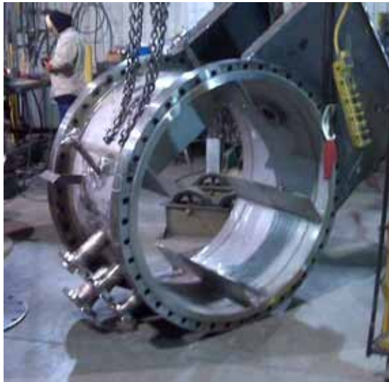
Evaporator Shell & Internal Seal Edges
