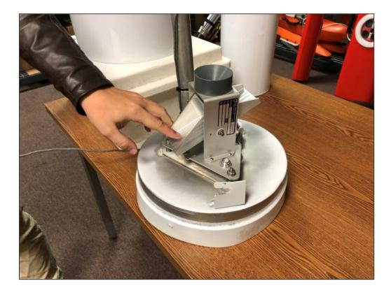
Close up of a tipping bucket rain gauge mechanism
