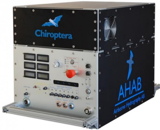
Figure 1: Leica AHAB Chiroptera.
