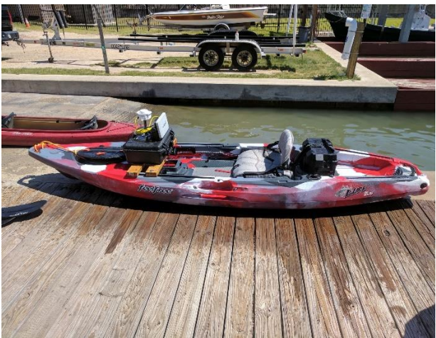
Figure 14: Kayak with sonar equipment.
