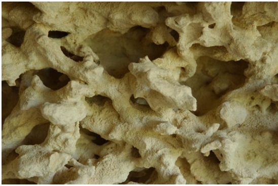
Groundwater occurs in both the matrix and the small conduits that have dissolved from the rock (both shown here).
