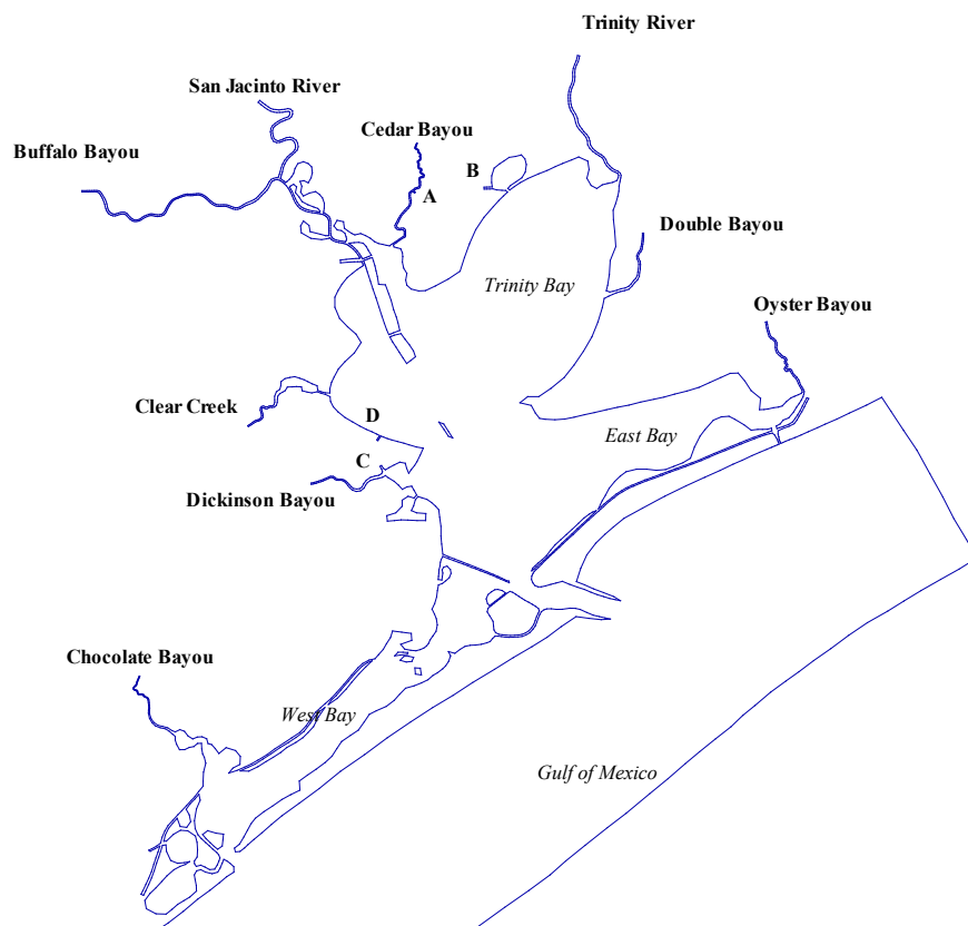
Figure 4. Nine TxBLEND inflow points, Oyster Bayou, Double Bayou, Trinity River, Cedar Bayou, San Jacinto River, Buffalo Bayou, Clear Creek, Dickinson Bayou, and Chocolate Bayou and four power plant intake and discharge sites including: A, intake site at Cedar Bayou; B, discharge site near upper Galveston Bay; C, intake site at Dickinson Bayou; D, discharge site near Bacliff.
